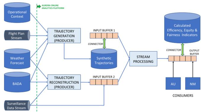
Fig. 2. A schematic of the AURORA real-time analytics platform.
